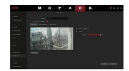
Step 2: Select the smart event alarm mode for setting the channel. Smart event alarms supported by the device include Human, Face, Face Comparison. Each smart detection can be configured with different alarm processing method.
